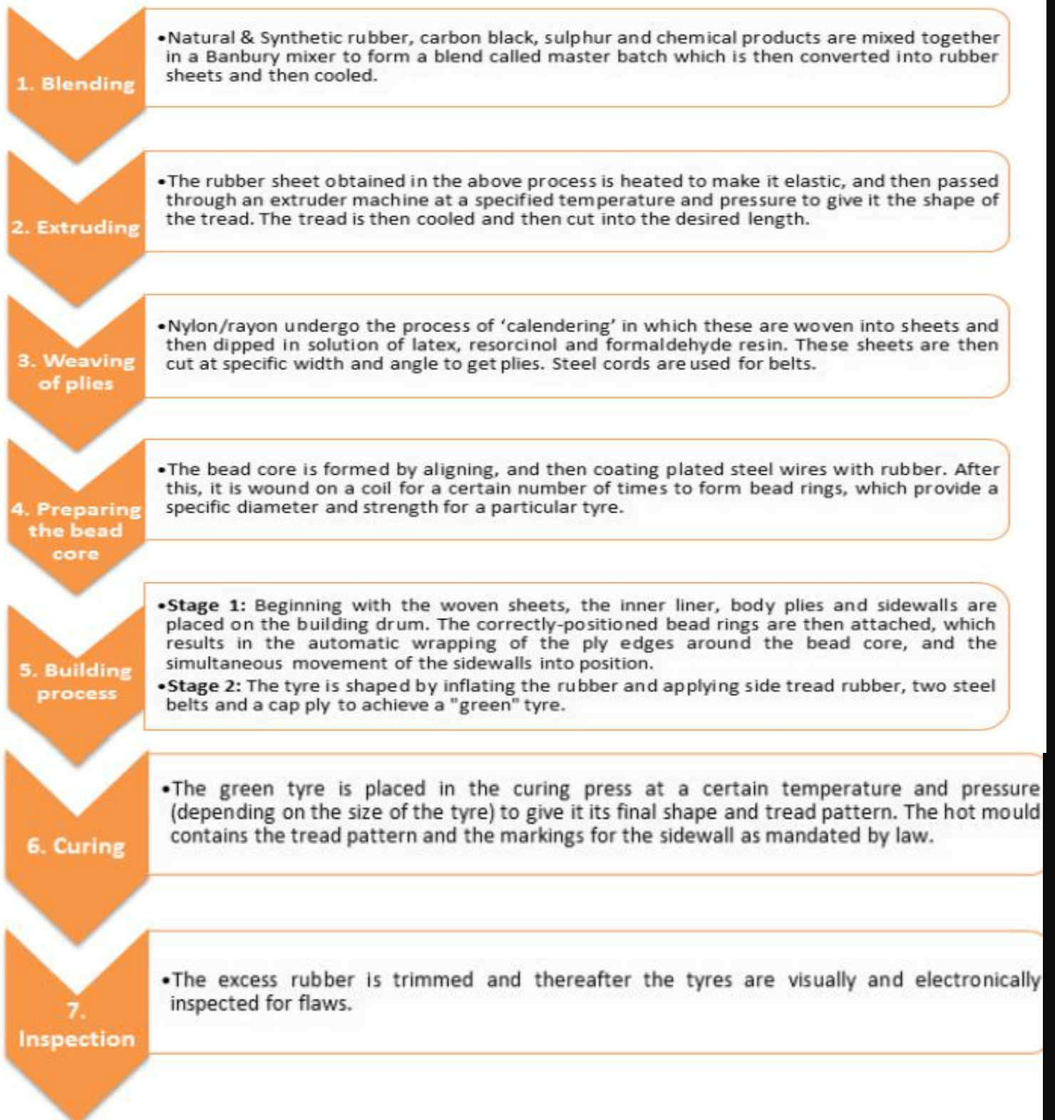
Chart 1: Tyre manufacturing process
